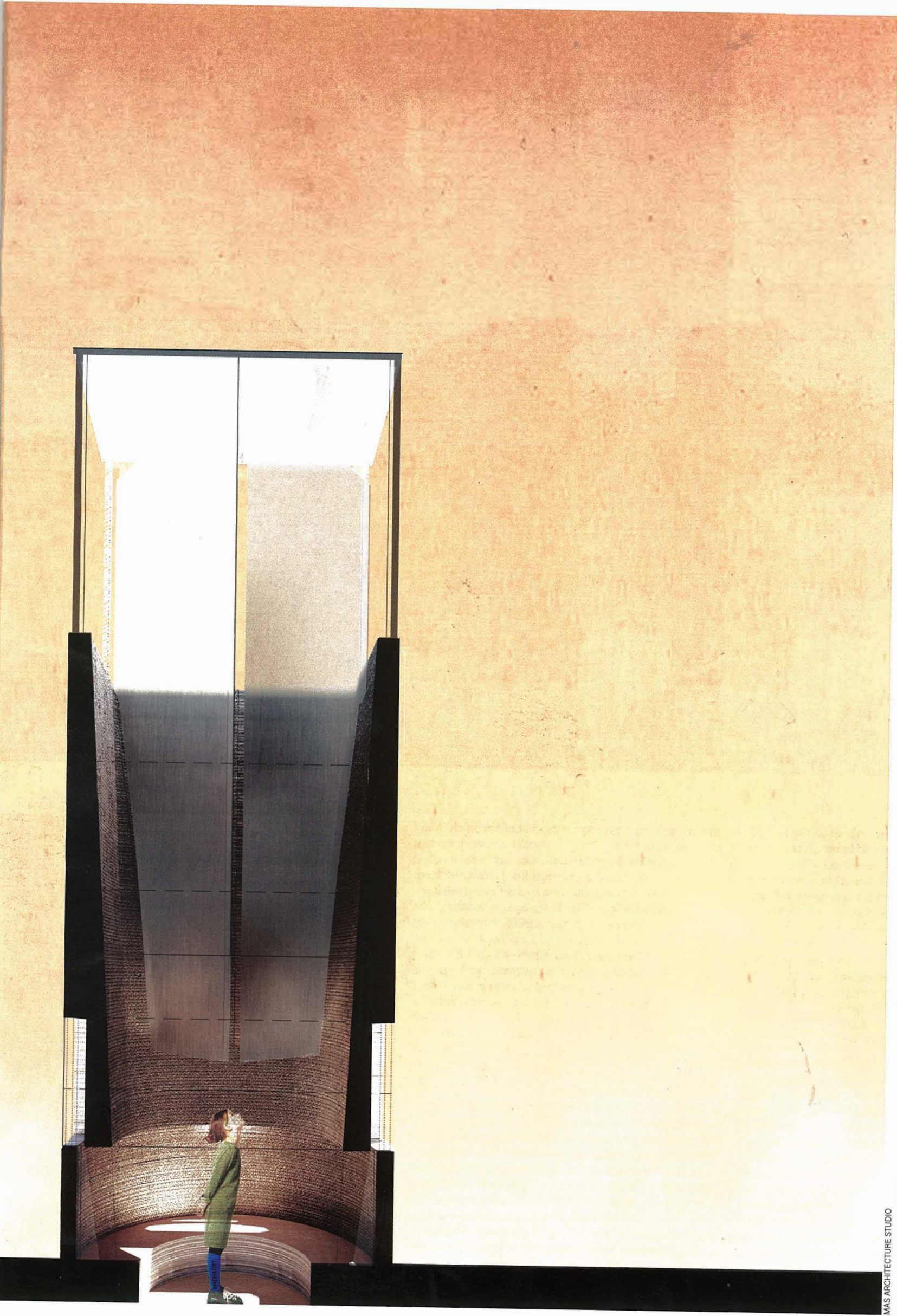
Crafted from recycled cardboard and unfinished aluminium, Barjeel offers a modern take on the traditional wind tower
